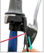
To lubricate the brake and shifter cables, apply a few drops of low viscosity oil to the cables. To expose some brake cable, visible from the front of the lever or the side on the e-Strider, squeeze the brake lever. To expose the shifter cable shift to gear 1 or on the e-Strider, shift to 4<sup>th</sup> gear, then pull the cable housing down a bit until the shifter cable is visible.
