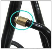
On the 8s and *e-Strider Pro*, lubricate the brass connector on the upper end of the strut with grease.
