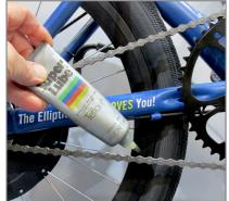
Use chain lubricant, DO NOT use a WD40 type water displacer.
