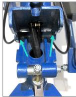
Lubricate the rear pivot of fold joint by adding a few drops of oil as shown.
