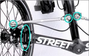
Lubricate the inboard and outboard spherical rod ends with grease and the king pin bolt bushings with low viscosity oil.
