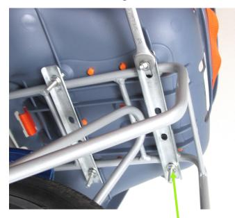
3. Set the Child Carrier on the luggage rack so that the carriage bolts straddle the top rail of the luggage rack on either side. Insert the brackets over the bolts and screw on the flange nuts. Tighten the nuts evenly side to side with a 10 mm open end wrench.
