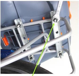
4. After the flange nuts have been tightened, screw on and tighten the nylon lock nuts with the 10 mm open end wrench.
