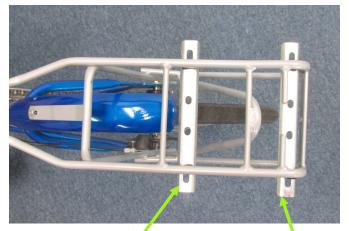
2. With the Child Carrier in place, the brackets under the top rail of the luggage rack will be as shown, with one bracket as far rearward as possible and the other bracket about 6" forward.
