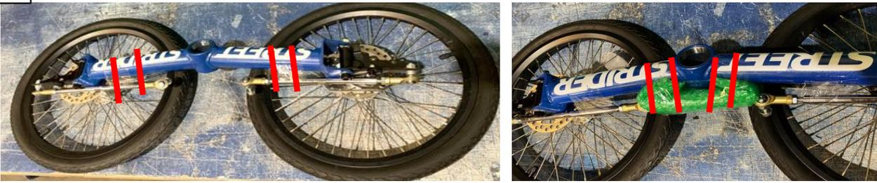
**G** Set the frame mid section on a box to wrap and tape, covering the front of the frame.
