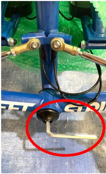
**B** With 13 mm or adjustable wrench, unscrew inboard rod end from lock nut inside bracket, replace nut onto rod end. When 2nd rod end is unscrewed, allow frame to roll onto side.
