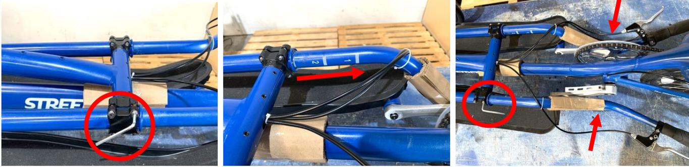
**E** With 5 mm wrench, loosen brake lever clamp, rotate levers toward wheel and re-tighten.
