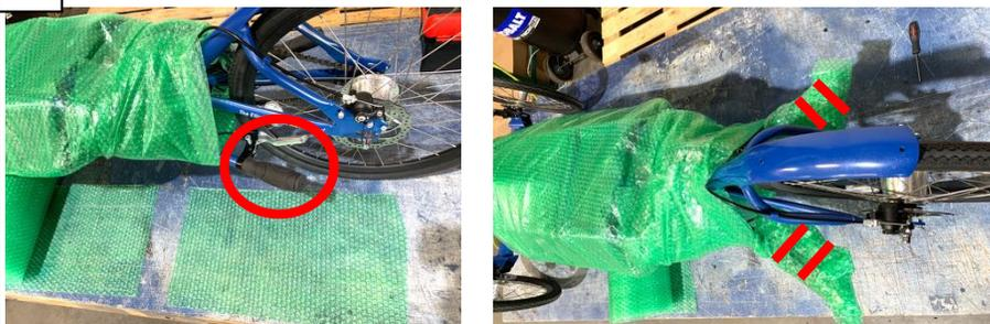
**C** Wrap and tape a piece of bubble cushion around fender, and finish with a wrap and tape around the brake levers and fender.
