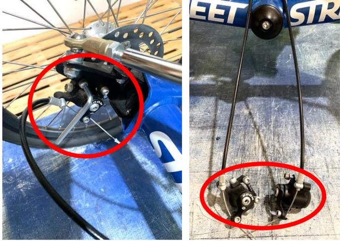
**B** Wrap and tape a short piece of bubble cushion around brakes and tuck them into the wrap around the front of the frame.
