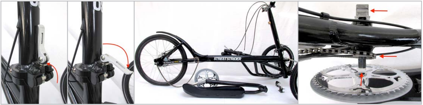
Figure 3.4.4 Rotate the QR stem to the vertical position so that the lever is against the head tube then close the lever downward.
