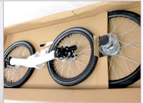
Figure 3.1.3 The front wheel assembly and rear wheel are the next 2 layers. Remove the wheels and set aside.
