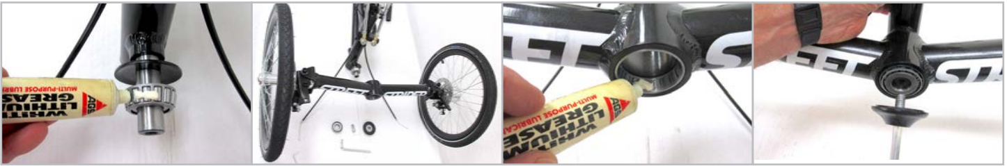
Figure 3.2.4 With the frame upright, slide the back plate and one of the tapered bearings, with taper facing forward, onto the shaft. Grease the bearings.
