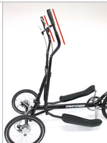
Figure 3.4.19 Attach the lower and upper pole on the left side following the procedure used on the right side. Make sure the left and right poles are set to the same height, rotate the poles to approximately shoulder width of the user and also parallel from the side view.
