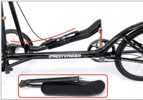
Figure 3.4.12 Place the left ski assembly on the left of the frame, rotate the right crank to the 12 o'clock position and rest the left upper pole on the right foot platform.
