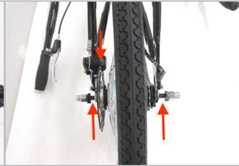
Figure 3.3.8 Unscrew acorn nuts on each end of the axle so there is an exposed section of axle under the non-turn washers that can slide into the dropouts. On the left side, align the brake rotor with the brake caliper gap.
