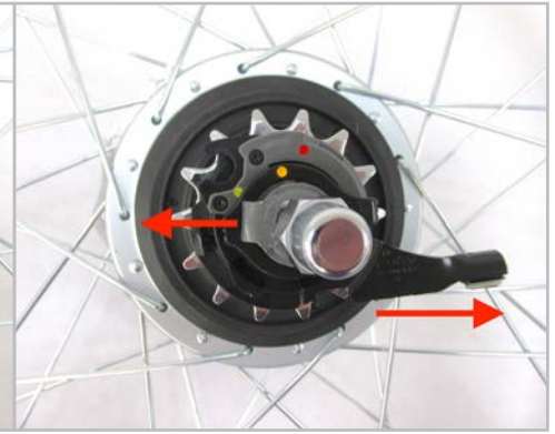
Figure 3.3.6 Replace the non-turn washer with tongue pointing rearward, and screw the acorn nut back onto the axle a few turns.
