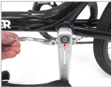
Figure 3.4.15 Slide the crank arm opening over the BB end piece as far as possible.
