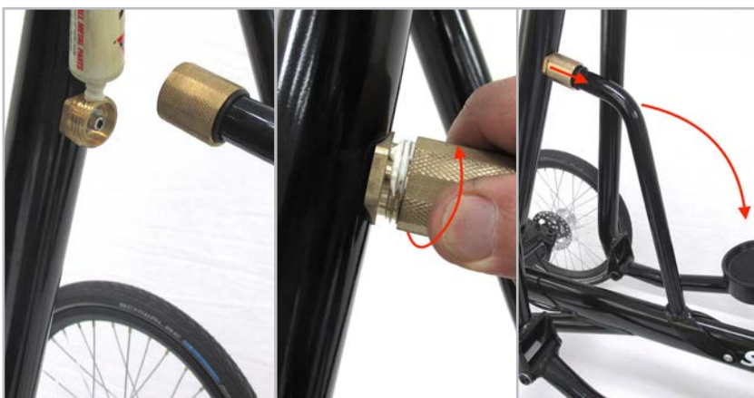
Figure 3.7.2 Add some grease to the threads of the brass receiver attached to the rear side of the head tube, press the brass collar over the receiver and tighten. To fold the head tube down the brass collar is disconnected from the receiver and the strut folded backwards pivoting at the saddle screw.
