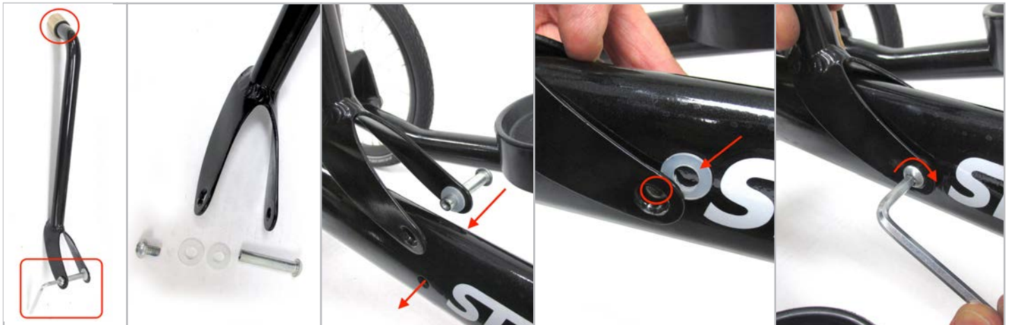
Figure 3.7.1 Retrieve the frame strut, which has a brass threaded collar at the top and frame saddle at the bottom. Using the 5 mm hex wrench, unscrew and separate the binding screw and the 2 nylon washers. Insert the longer female end of the screw through the hole at the end of the right side of the saddle and add a nylon washer on the inner side of the saddle. Align the saddle and screw with the frame hole and push the screw through the hole until it appears in the frame hole on the left side. Slide the second nylon washer between the saddle and the frame and over the screw end. Insert the male screw and tighten the screw with the 5 mm hex wrench. the receiver and tighten.
