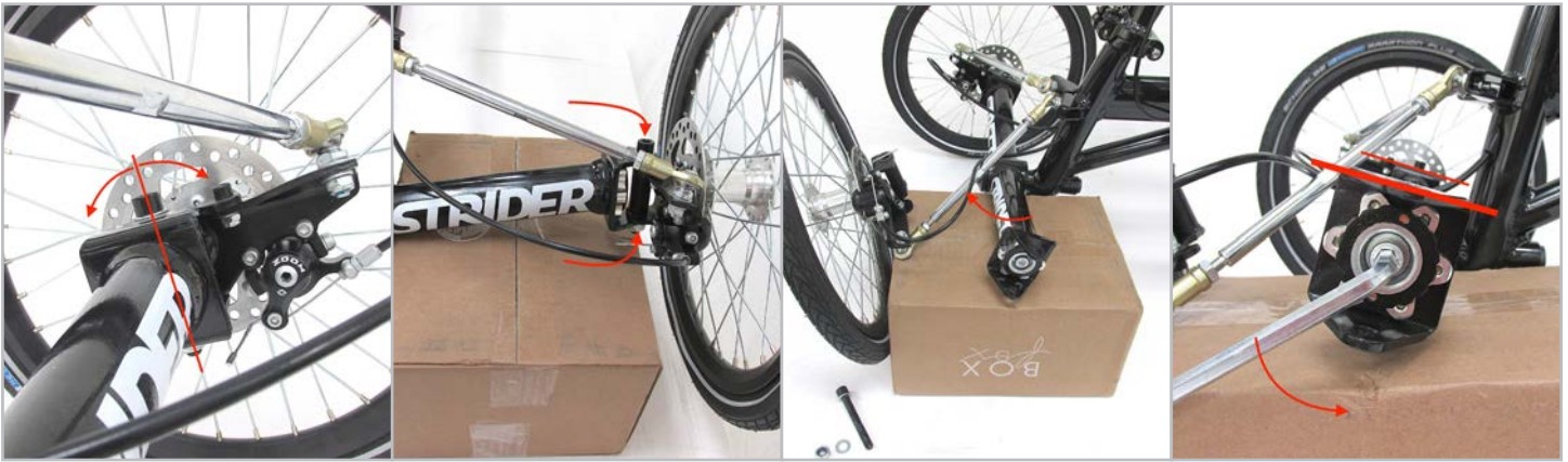
Figure 3.9.2 The caster angle of the King Pin can be set at lower or higher values.
