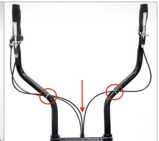
Figure 3.4.20 Rotate the brake levers to a forward position, rotate the shifter so the gear indicator window is seen by the user, tighten the brake lever clamps with the 5 mm hex wrench and the shifter clamp with the 3 mm hex wrench. Use 2 of the zip ties to orderly hold the cables to the poles.
