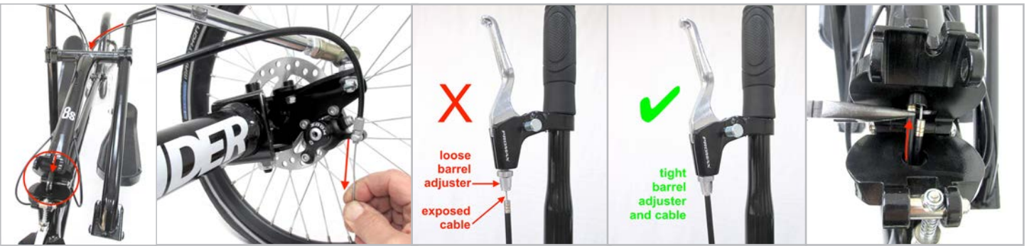
Figure 3.5.2 Fold the head tube down and push the cable housing from the left brake lever into the opening at the top of the crossbar so that the base of the cable doubler is visible through the hole in the fold joint. While pulling the cable down at the caliper make sure there is no exposed cable visible at the brake lever by inserting the cable housing ferrules into the brake lever barrel adjuster. Also, insert the cable housing ferrules into the base of the cable doubler using the pliers if needed.
