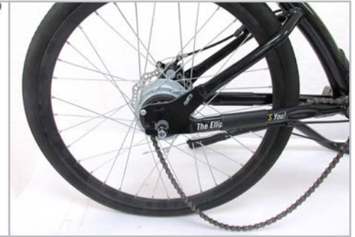
Figure 3.3.9 Slide axle into dropouts all the way forward, align the tongue of the non-turn washers with dropout slots, finger tighten the acorn nuts on both ends, and loop chain around hub sprocket.
