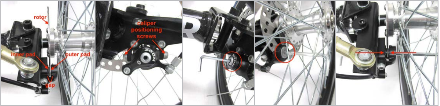
Figure 3.5.1 Make sure the brake rotor is centered in the caliper gap between the pads and the wheel spins freely. If adjustment is needed, loosen the caliper positioning screws with a 5 mm hex wrench, tighten the inner pad with the 3 mm hex wrench, inserted through the caliper lever, and the outer pad with the 5 mm hex wrench to center the rotor in the gap, then tighten the positioning screws. If the rotor is already centered in the caliper gap tighten the pads against the rotor in order to attach the brake cable in the next steps.
