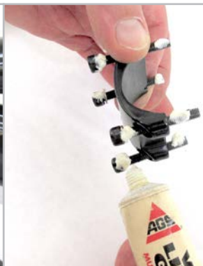
Figure 3.4.2 Apply a little grease to the screw heads and threads then set the caps with screws on the table.
