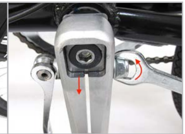
Figure 3.4.18 If the QR lever closes without any resistance open the lever, pull the crank arm off the BB ¼ inch (6 mm), tighten the 17 mm stem nut ¼ turn, push the crank arm back on, and close the QR lever. If needed, repeat until QR closes with some resistance.
