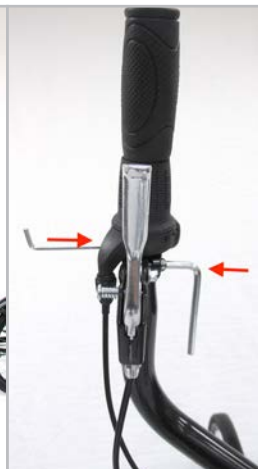
Figure 3.4.20 Rotate the brake levers to a forward position, rotate the shifter so the gear indicator window is seen by the user, tighten the brake lever clamps with the 5 mm hex wrench and the shifter clamp with the 3 mm hex wrench. Use 2 of the zip ties to orderly hold the cables to the poles.
