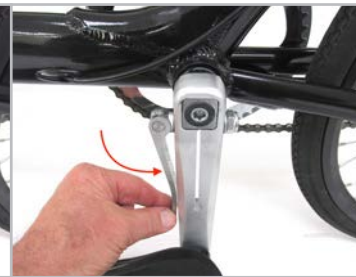
Figure 3.4.17 Close the QR lever against the crank arm.
