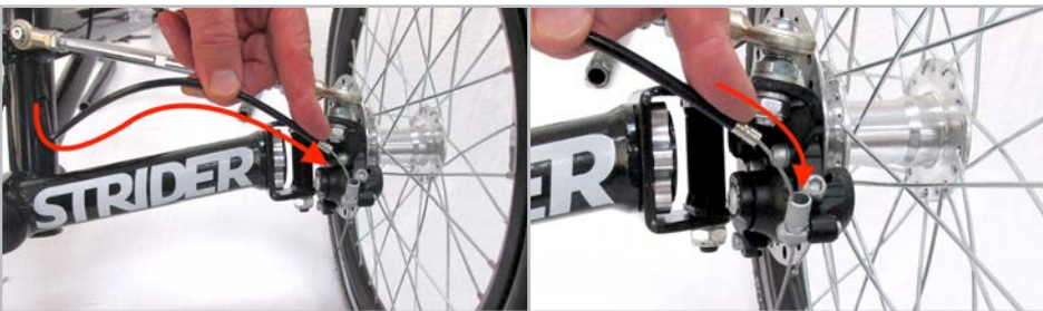
Figure 3.2.11 Route the front brake cables from the head tube, under the steering linkage and over the front beam. If the cable housing is off of the cables slide it back on. Insert the left and right cable and housing into the barrel adjuster on the left and right brakes, respectively.
