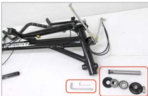
Figure 3.2.1 Lay the frame on it's left side. Retrieve the front beam shaft assembly, take the cap, tapered bearings and back plate off the shaft, and get the 8 and 3 mm hex wrenches.
