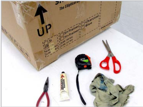
Figure 3.1.1 The StreetStrider box shows which side is up. You will need a blade or scissors, pliers, tape measure, grease and a rag.
