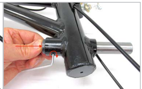
Figure 3.2.3 With the shaft inserted all the way forward, secure the shaft by tightening the set screw with the 3 mm hex wrench.
