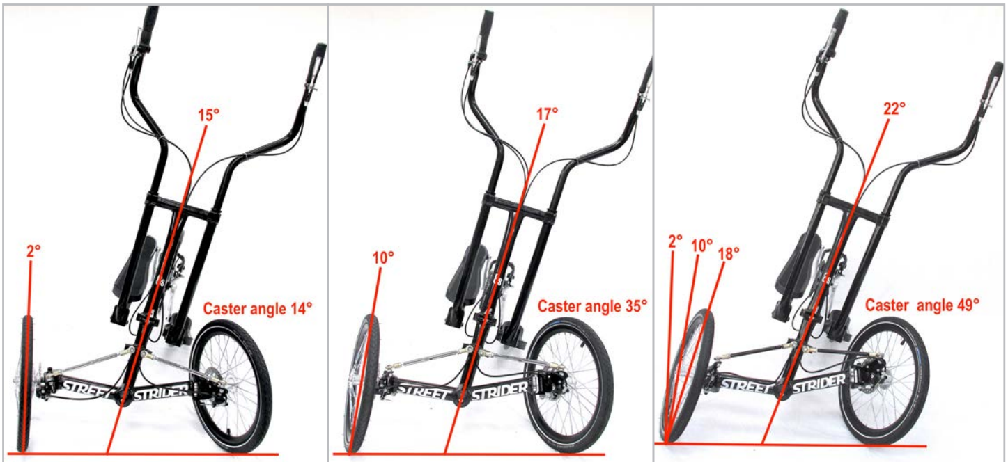
Figure 3.9.1 By setting the caster angle at 14° the StreetStrider frame can lean about 15° but the outer front wheel will only camber about 2°. Most of the steering results form a change in toe angle. At 35° caster angle the frame leans about 17° and the outer wheel has more camber to about 10°. At 49° caster angle the lean increases to 22° and the outer front wheel cambers to 18°. In a turn, the inner wheel toe angle and camber lean is a bit more than the outer wheel.
