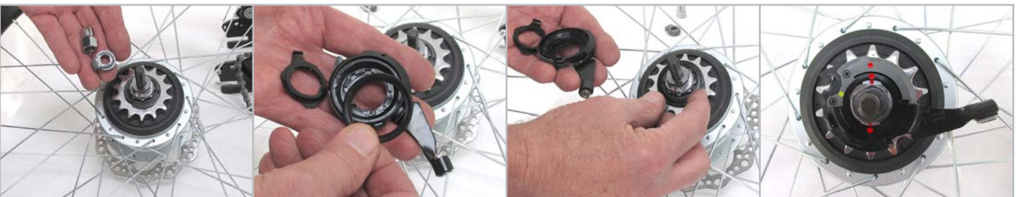
Figure 3.3.1 Remove the silver acorn nut and gray (or yellow) non-turn washer from the right axle end.
