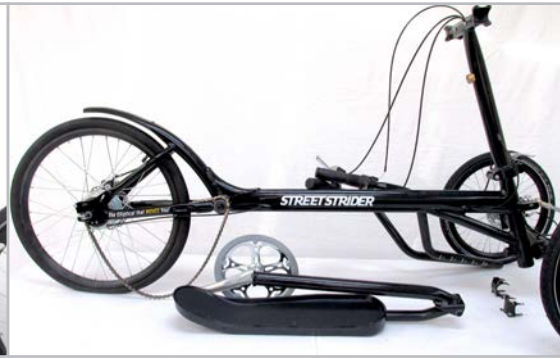
Figure 3.4.5 Retrieve the right foot platform assembly (lower pole, ski, foot platform, and crank arm with chain ring) and position next to right side of the frame. Make sure the chain is looped over the BB spindle.
