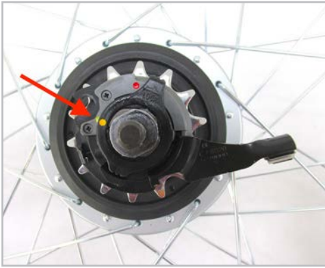
Figure 3.3.4 Put the lock ring onto the cassette pulley so that the 2 yellow dots are adjacent.
