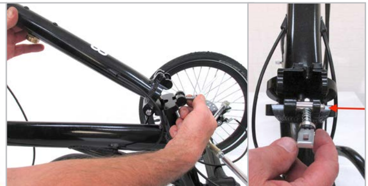
Figure 3.4.3 Raise the head tube while sliding the quick release, QR, clamp pin to the right. With the head tube in the full upright position allow the clamp pin to insert into the hole.
