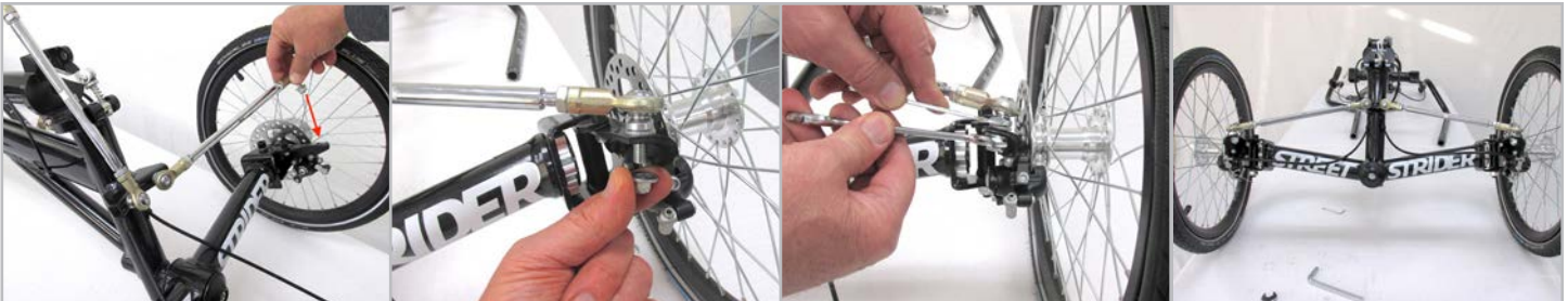
Figure 3.2.8 Lower the left steering linkage so the outboard rod end can be attached to the left steering knuckle.
