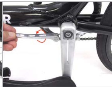
Figure 3.4.16 Rotate the QR lever 180° so that the QR stem fits into the BB end piece channel.
