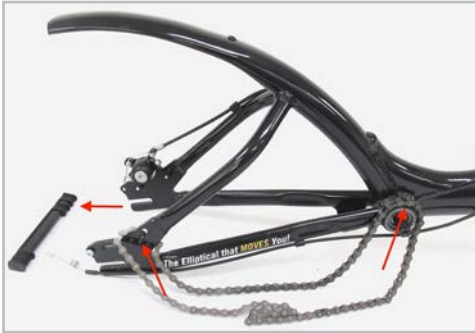
Figure 3.3.7 Remove the plastic brace in the rear drop and loop the chain over the rear drop out and the bottom bracket, BB.
