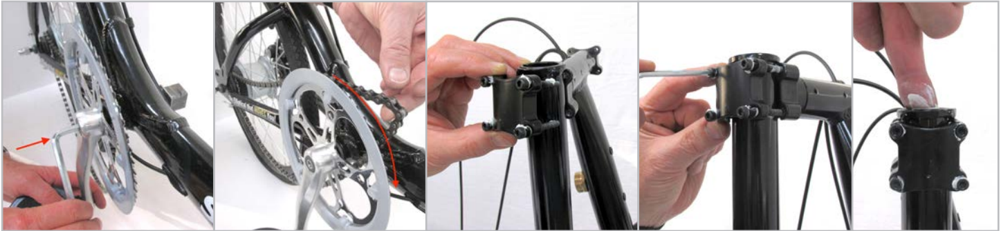
Figure 3.4.7 Lift the right crank arm so it is in the 6 o'clock position and insert it onto the BB square spindle. Using the 8 mm hex wrench, screw the crank bolt into the spindle and tighten to 30 ft lb, then wrap the chain around the chain ring.
