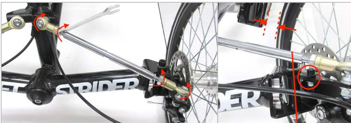
Figure 3.8.3 When the wheels are parallel to within 1/8" or 3 mm, tighten the jam nuts against the rod ends. To tighten the jam nuts, first rotate both rod ends as far as possible in the direction that the jam nuts will tighten, then use the 14 mm wrench to tighten the jam nut against the rod end. Check to make sure that each steering linkage rod is free to rotate as the StreetStrider is leaned to each side.
