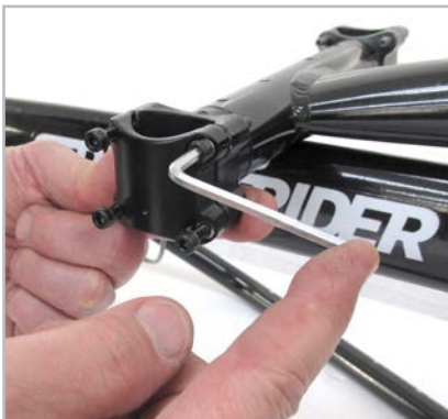
Figure 3.4.1 While the head tube is folded onto the main frame, use the 4 mm hex wrench to remove the 4 screws and caps from the both pole clamps at Joint #1.
