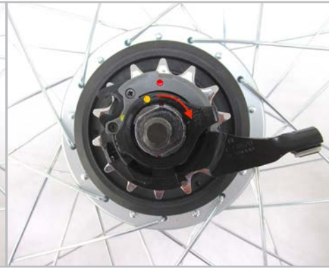
Figure 3.3.5 Rotate the lock ring 45° clockwise to lock the cassette pulley onto the hub.
