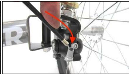
**Figure 3.2.11** Route the front brake cables from the head tube, under the steering linkage and over the front beam. If the cable housing is off of the cables slide it back on. Insert the left and right cable and housing into the barrel adjuster on the left and right brakes, respectively.
