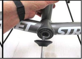
**Figure 3.2.7** Insert the beam and other bearing onto the shaft with the taper facing rearward. Put the cap over the front of the beam shaft, insert the 10 mm screw, and tighten with the 8 mm hex wrench.
