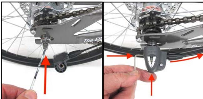
**Figure 3.6.1** Retrieve the 3i shifter push rod from the parts pack, apply a little grease to the rod, and insert it into the hole on the right end of the axle, black end first. Attach the bell crank to the right axle by fitting it over the push rod and right axle nut as close to the drop out as possible, with the shifter cable routed along the lower edge of the frame chain stay, then securing it by tightening the 2.5 mm set screw with the 2.5 mm hex wrench.
