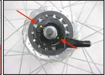
**Figure 3.3.6** Place the cassette pulley over the axle so that the yellow dots on the washer and the cassette pulley are in line.
