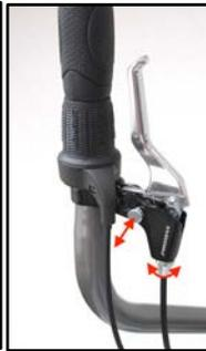
**Figure 3.5.6** Both brake levers have a parking brake pin to hold the brake lever in a squeezed position. If the parking brake does not hold, unscrew the brake lever barrel adjuster.
