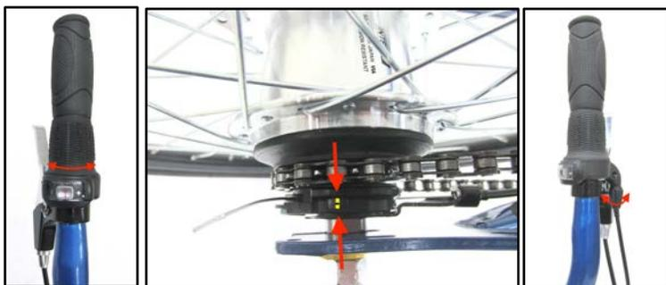
**Figure 3.6.6** To check gear alignment, twist the shifter to gear 4 and make sure the 2 yellow lines in the cassette pulley window are in line. If the lines are offset use the barrel adjuster nut at the shifter to move the lines into the correct position.
