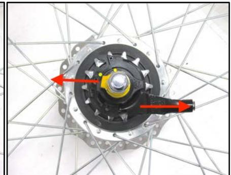
**Figure 3.3.9** Replace the non-turn washer with tongue pointing rearward, and screw the acorn nut back onto the axle a few turns.
