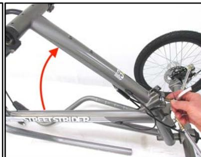
**Figure 3.4.3** Raise the head tube while sliding the quick release, QR, clamp pin to the right. With the head tube in the full upright position allow the clamp pin to insert into the hole.
