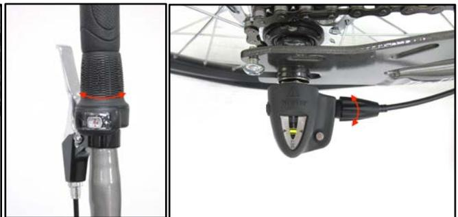
**Figure 3.6.2** Set the twist grip shifter to gear 2. On the bell crank, make sure the interior thicker yellow line under the gear alignment window is between the two thinner yellow lines on the window. If needed, use the shifter cable barrel adjuster at the front of the bell crank to move the interior line to the correct gear 2 position.
