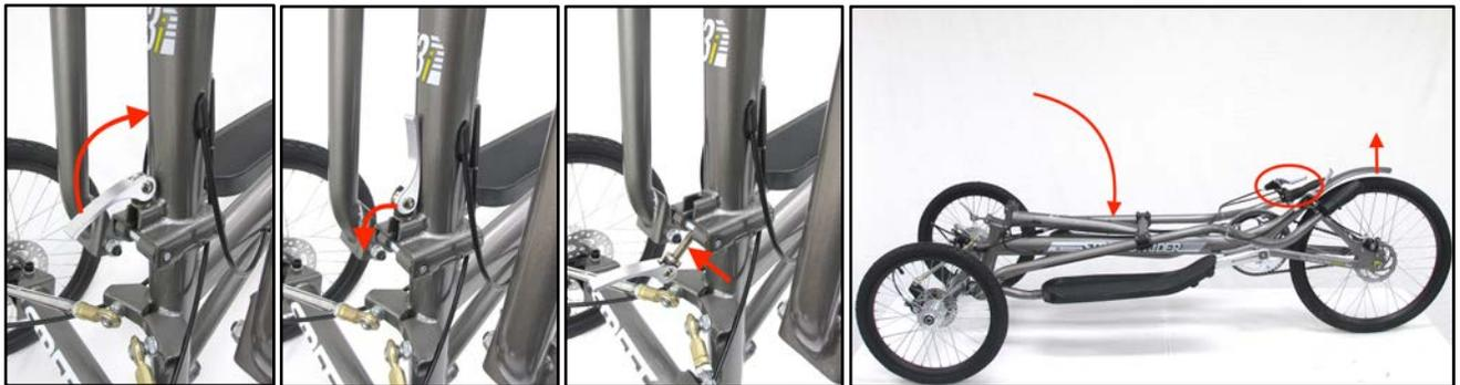
**Figure 3.8.4** Lift the QR lever of the head tube fold joint up and rotate the stem forward. With one hand supporting the head tube, pull the QR stem to the right side so the pin disengages from the hole and lower the head tube down. With the rear brake locked the strider can be lifted by the rear fender and rolled or stood up against a wall for storage.
