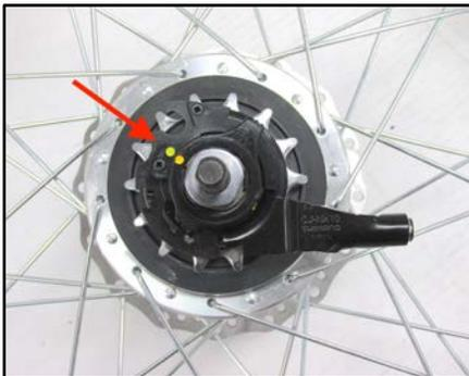
**Figure 3.3.7** Put the lock ring onto the cassette pulley so that the 2 yellow dots are adjacent.
