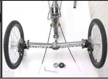
**Figure 3.2.5** Unfold the front wheels on the front beam and set the front wheel assembly in front of the shaft.
