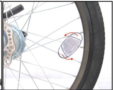
**Figure 3.5.7** To install the 3 wheel reflectors onto the spokes, position the reflector between spokes and rotate so the reflector ends snap around the spokes.
