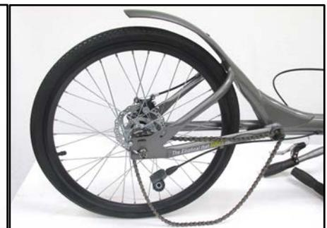
**Figure 3.3.3** Slide axle into dropouts all the way forward, align the tongue of the non-turn washers with dropout slots, finger tighten the axle nuts on both ends, and loop chain around hub sprocket.
