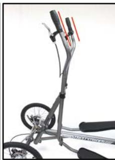
**Figure 3.4.19** Attach the lower and upper pole on the left side following the procedure used on the right side. Make sure the left and right poles are set to the same height, rotate the poles to approximately shoulder width of the user and also parallel from the side view.
