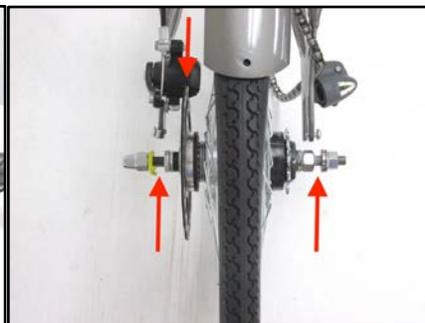
**Figure 3.3.2** Unscrew acorn nuts on each end of the axle so there is an exposed section of axle under the non-turn washers that can slide into the dropouts. On the left side, align the brake rotor with the brake caliper gap.
