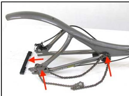
**Figure 3.3.1** Remove the plastic brace in the rear drop and loop the chain over the rear drop out and the bottom bracket, BB.
