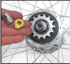
**Figure 3.3.4** Remove the silver acorn nut and yellow (or gray) non-turn washer from the right axle end.
