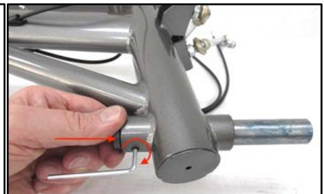
**Figure 3.2.3** With the shaft inserted all the way forward, secure the shaft by tightening the set screw with the 3 mm hex wrench.
