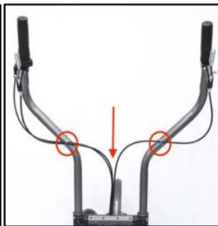
**Figure 3.4.20** Rotate the brake levers to a forward position, rotate the shifter so the gear indicator window is seen by the user, tighten the brake lever clamps with the 5 mm hex wrench and the shifter clamp with the 3 mm hex wrench. Use 2 of the zip ties to orderly hold the cables to the poles.
