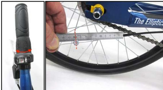
**Figure 3.6.3** At the grip on the right pole, twist the shifter to gear 1. At the rear hub, pull the shifter cable taut and make sure the length of cable from the ferrule to the center of the clamping screw is 101 mm (4 in). If not, loosen the nut with the 10 mm wrench, adjust to 101 mm and tighten.
