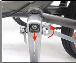
**Figure 3.4.18** If the QR lever closes without any resistance open the lever, pull the crank arm off the BB ¼ inch (6 mm), tighten the 17 mm stem nut ¼ turn, push the crank arm back on, and close the QR lever. If needed, repeat until QR closes with some resistance.
