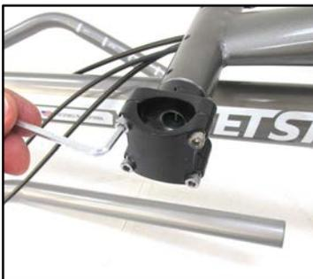
**Figure 3.4.1** While the head tube is folded onto the main frame, use the 4 mm hex wrench to remove the 4 screws and caps from the pole clamps at Joint #1.
