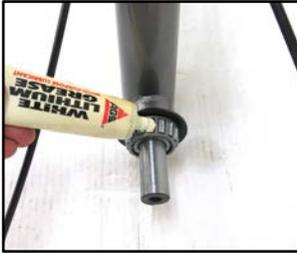
**Figure 3.2.4** With the frame upright, slide the back plate and one of the tapered bearings, with taper facing forward, onto the shaft. Grease the bearings.
