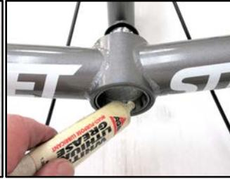
**Figure 3.2.6** Grease the front bearing race in the front beam.
