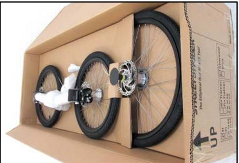
**Figure 3.1.3** The front wheel assembly and rear wheel are the next 2 layers. Remove the wheels and set aside.
