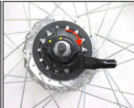
**Figure 3.3.8** Rotate the lock ring 45° clockwise to lock the cassette pulley onto the hub.
