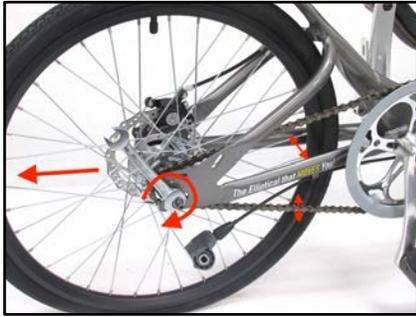
**Figure 3.5.4** With the chain wrapped around both the right crank arm chainring and the rear hub sprocket, pull the rear wheel backwards to make the chain taut, center the front of the wheel in the frame chain stays, and tighten the axle nuts with the 15 mm wrench, first right side then left. A taut chain should only move about ½" if lifted at a point midway between the chain ring and hub sprocket.
