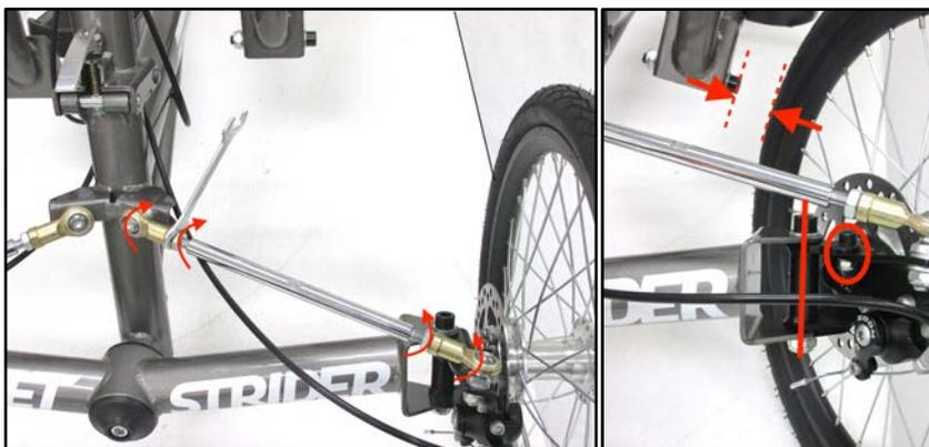
**Figure 3.7.3** When the wheels are parallel to within 1/8" or 3 mm, tighten the jam nuts against the rod ends. To tighten the jam nuts, first rotate both rod ends as far as possible in the direction that the jam nuts will tighten, then use the 14 mm wrench to tighten the jam nut against the rod end. Check to make sure that each steering linkage rod is free to rotate as the *StreetStrider* is leaned to each side.
