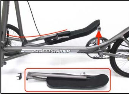
**Figure 3.4.12** Place the left ski assembly on the left of the frame, rotate the right crank to the 12 o'clock position and rest the left upper pole on the right foot platform.
