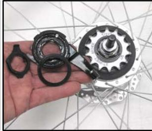
**Figure 3.3.5** From the parts bag retrieve the shifter cassette parts, the cassette pulley, the driver cap ring (often in the rear side of the pulley), and the lock ring. Press the driver cap over the hub driver until it snaps down.
