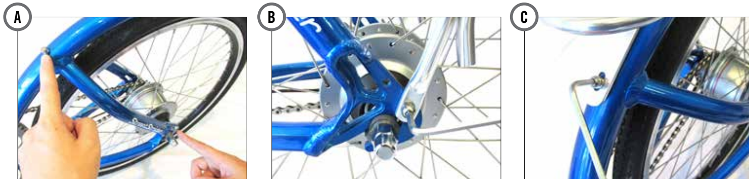
Figure 3-17. Installing the rear rack
