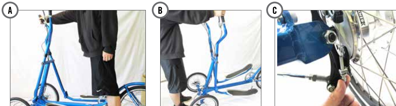
Figure 3-15. Checking brake function
