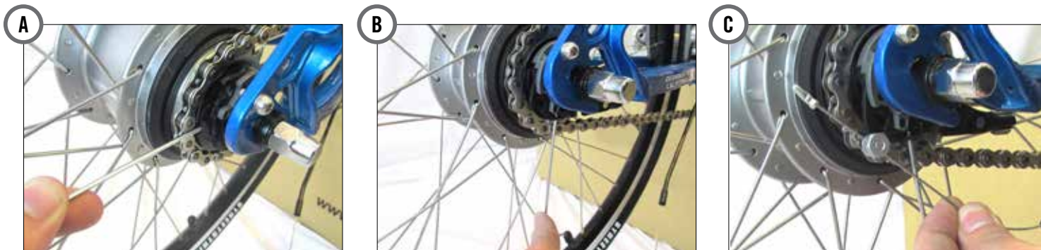
Figure 3-11. Installing the rear wheel (cont.)
