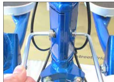
Figure 3-7. Unfolding the head tube
