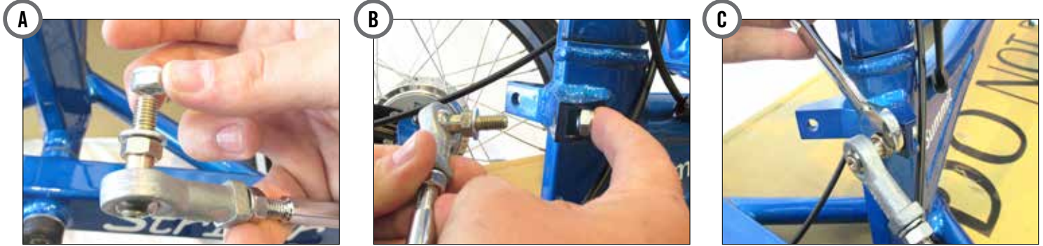
Figure 3-4. Attaching the two front wheels (cont.)
