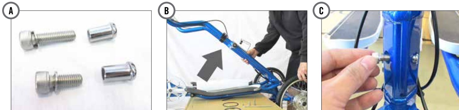
Figure 3-6. Unfolding the head tube
