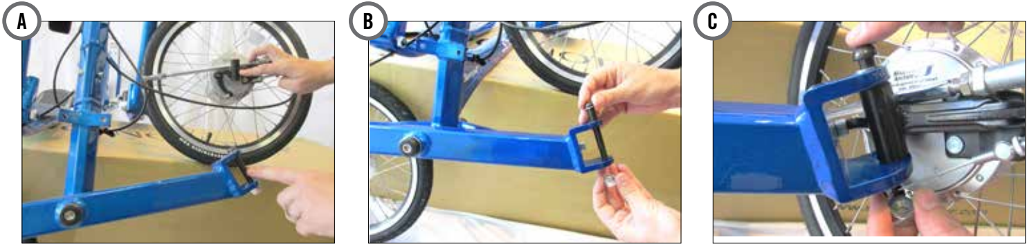
Figure 3-3. Attaching the two front wheels
