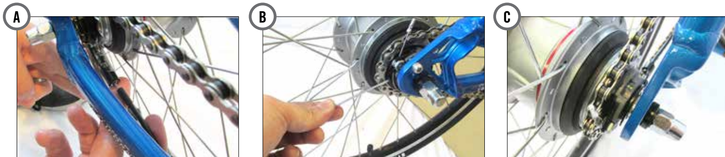
Figure 3-12. Installing the rear wheel (cont.)
