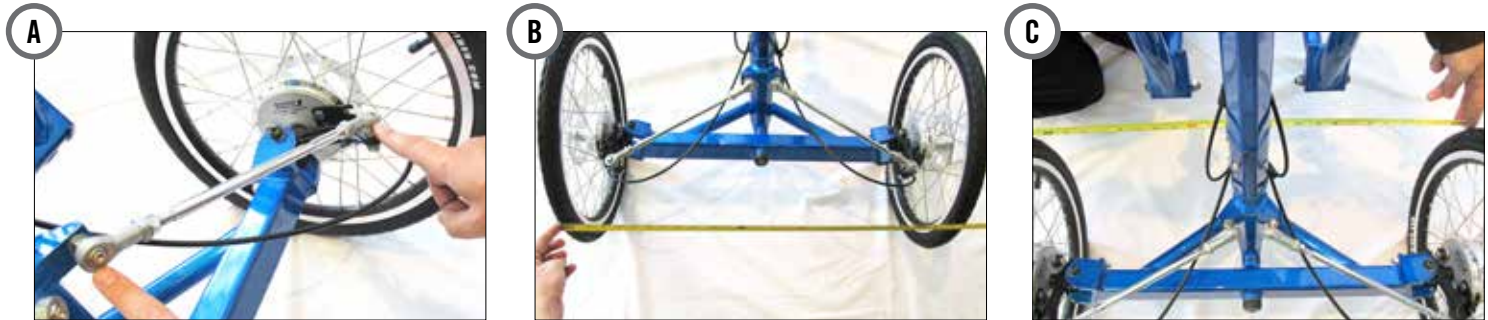
Figure 3-14. Aligning the front wheels
