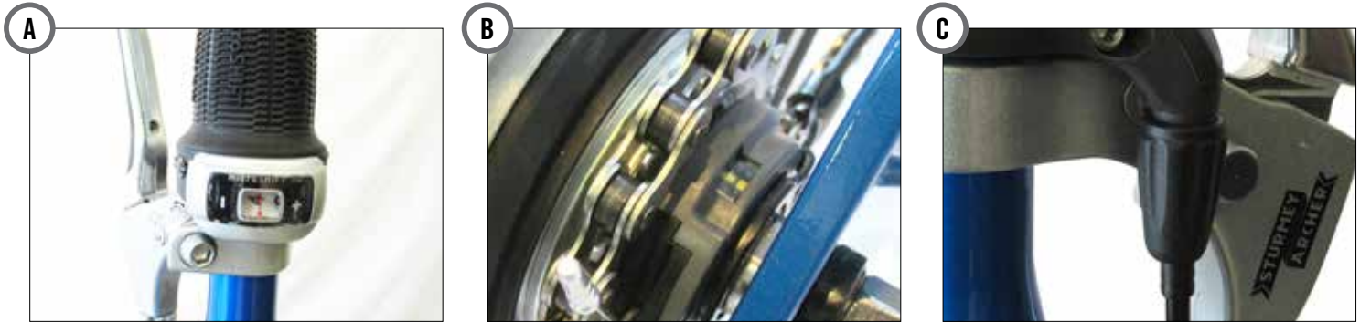
Figure 3-16. Adjusting the rear hub shifter
