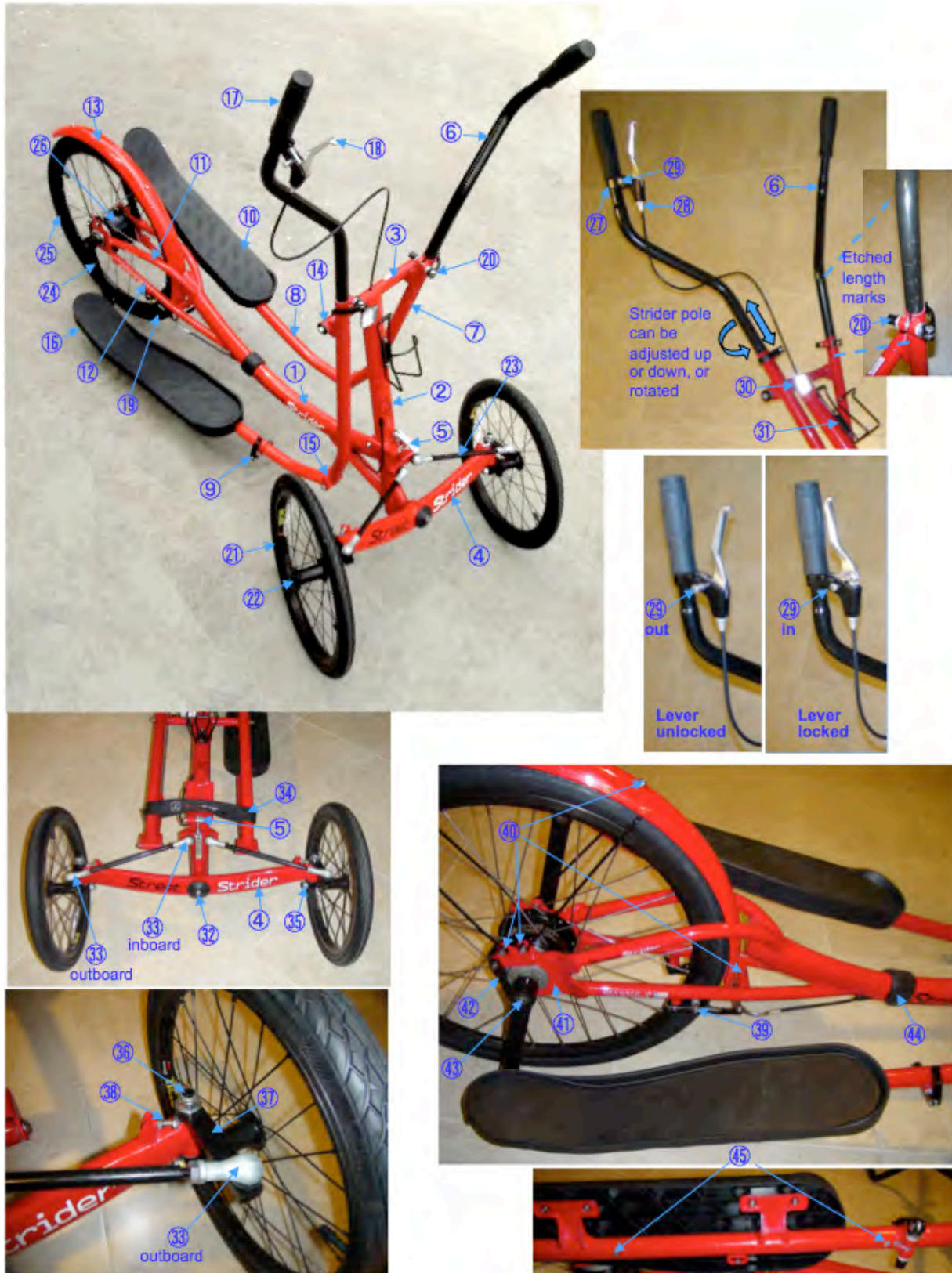
Figure 2A-1. StreetStrider Eclipse Parts. Refer to Table 2A-1 for part numbers and descriptions.
