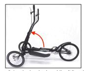
Raise the head tube while sliding the quick release (QR) clamp T-pin to the right. With the head tube in the full upright position, allow the QR clamp T-pin to insert into the hole. Rotate the QR stem to the vertical position so that the lever is against the head tube, then close the lever downward.
