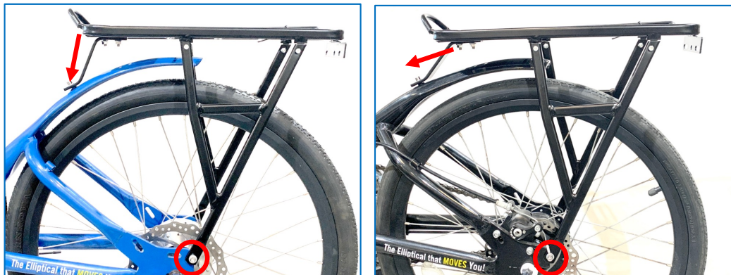
Figure 4. Attach the end of the legs to the threaded holes near the rear edge of the drop outs with an M5 screw on each side, then raise the rack up and forward to determine if the brace reaches the threaded hole in the fender. The steel frame fender on the StreetStrider 3i and 7i models has a lower profile than the aluminum frame on the StreetStrider 8s and 11s models, and this difference may require you to bend the brace forward to reach the threaded fender hole on the aluminum frame. With the brace positioned over the threaded hole in the fender, secure with an M5 screw.
