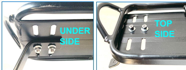
Figure 3. Attach the brace to the front of the top with two of the M5 screws, washers and nuts using a 4 mm hex wrench in the screw head and a 10 mm open end wrench on the nut.
