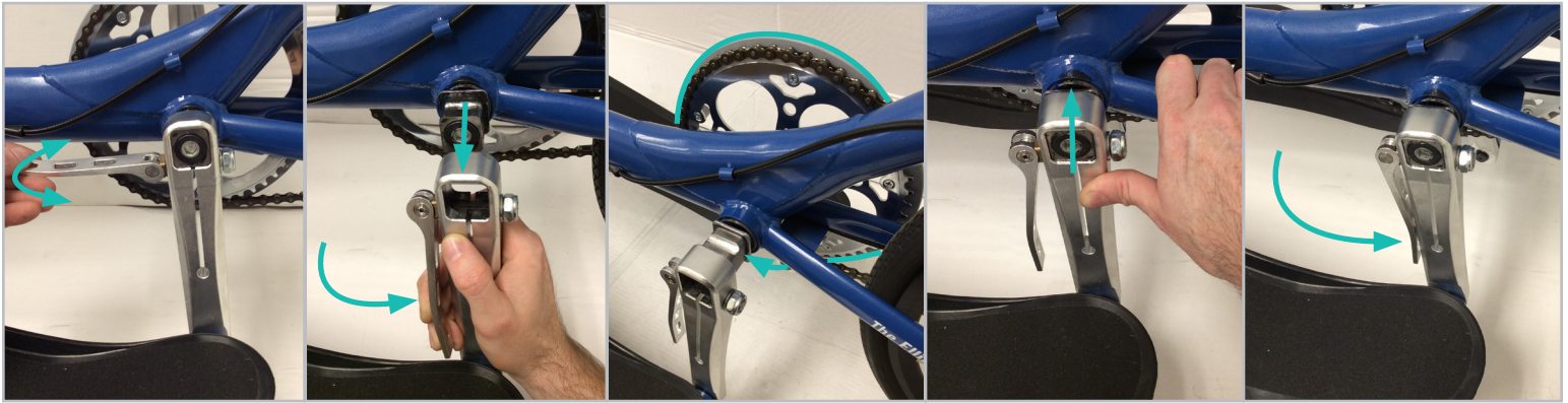
FIGURE 3.9.1 Stabilize the StreetStrider by engaging the right parking brake pin to lock the rear brake. From the left side of the StreetStrider, rotate the left crank arm to the 6 o'clock position, lift the quick release lever, rotate the lever 180° and lower it to the left side of the crank arm. Pull the crank arm off the BB block just to where the crank arm clears the block. Rotate the right crank down to the 6 o'clock position. Insert the crank arm over the end piece, lift the QR lever and rotate 180° then push the lever back down the side of the crank arm. Rotate the crank arms forward so the foot platforms are horizontal.
