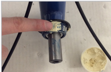
FIGURE 3.2.4 With the frame upright, slide the back plate and one of the tapered bearings, with taper facing forward, onto the shaft. Grease the bearings.
