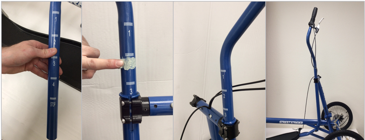
FIGURE 3.4.13 Apply a small amount of the included grit paste to the upper right pole - the pole with the brake lever and a shifter - at the height where the pole will be clamped. Then slide it into the lower pole to the level that fits the height of the user. The upper pole can also be rotated toward the side to provide a comfortable width for the user.
