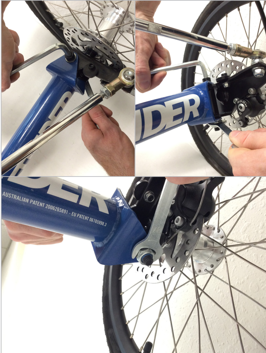
FIGURE 3.8.1 To adjust the stability of your StreetStrider, you can tighten or loosen the kingpin bolts on the Front Beam Assembly on both the left and the right steering knuckles. Using the 8 mm hex wrench for the kingpin bolt and a 17 mm open end wrench for the nut, tighten or loosen to adjust the stability to preference.
