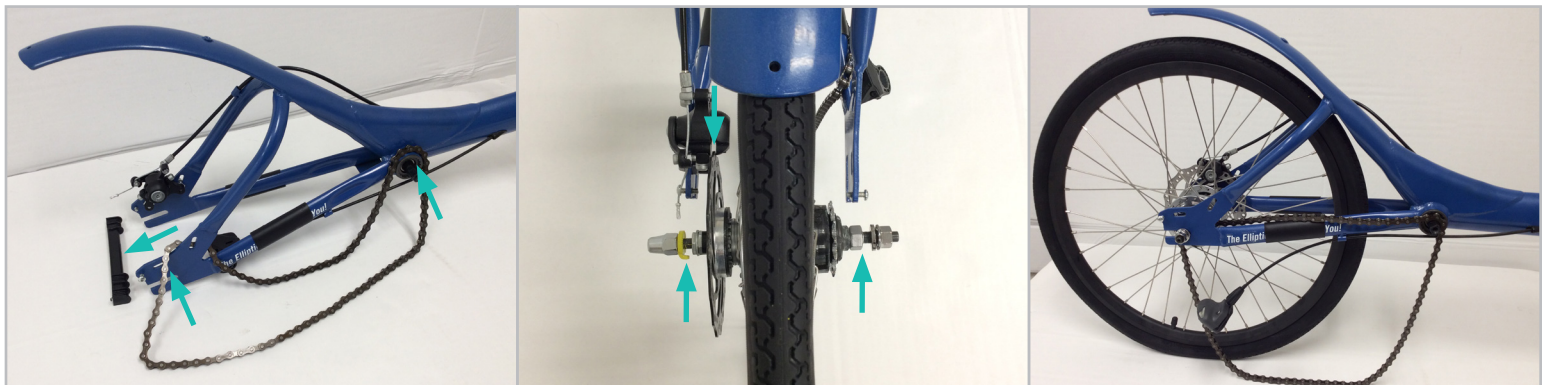
FIGURE 3.3.1 Remove the plastic brace in the rear dropout and loop the chain over the rear dropout and the bottom bracket, BB.
