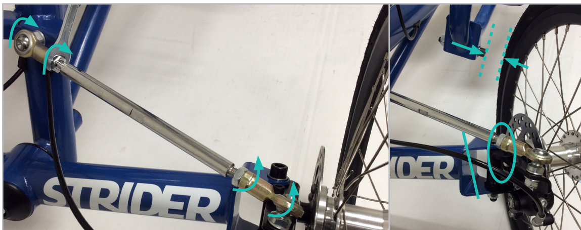
FIGURE 3.7.3 When the wheels are parallel to within 1/8" or 3 mm, tighten the jam nuts against the rod ends. To tighten the jam nuts, first rotate both rod ends as far as possible in the direction that the jam nuts will tighten, then use the 14 mm wrench to tighten the jam nut against the rod end. Check to make sure that each steering linkage rod is free to rotate as the StreetStrider is leaned to each side.
