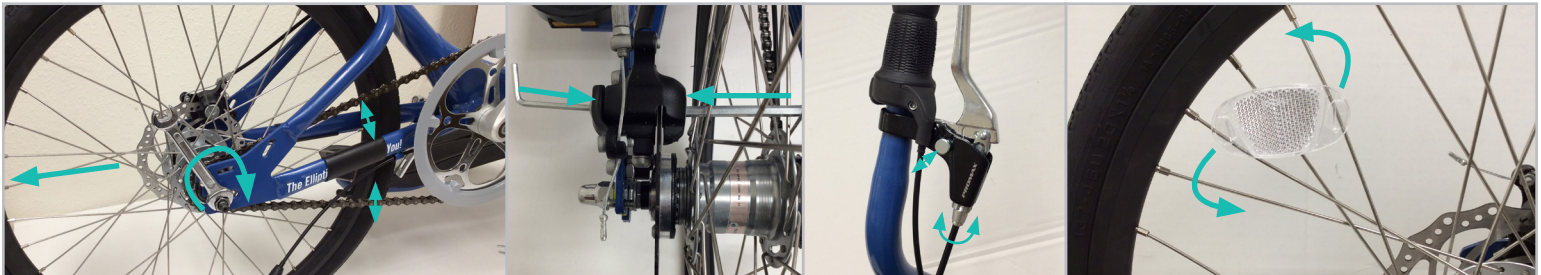
FIGURE 3.5.4 With the chain wrapped around both the right crank arm chainring and the rear hub sprocket, pull the rear wheel backwards to make the chain taut, center the front of the wheel in the frame chain stays, and tighten the axle nuts with the 15 mm wrench, first right side then left. A taut chain should only move about ½" if lifted at a point midway between the chain ring and hub sprocket.
