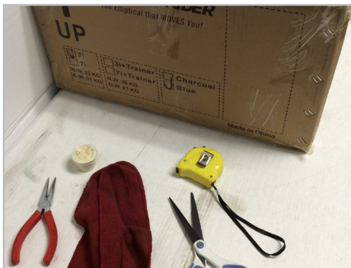
FIGURE 3.1.1 The StreetStrider box shows the up direction. You will need scissors or blade, pliers, tape measure, grease and rag.
