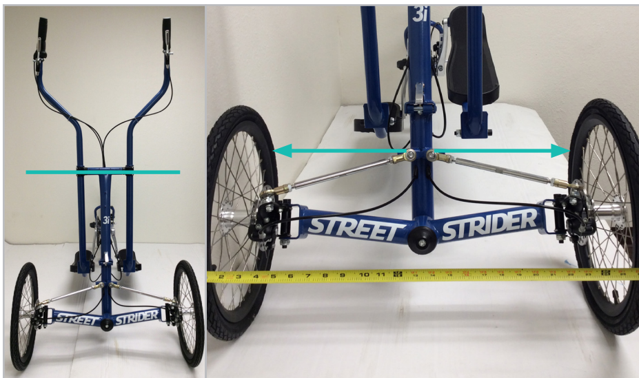
FIGURE 3.7.1 The front wheels should be aligned/parallel so they do not point in (toe in) or point out (toe out). Alignment is important for performance so take the time to do it correctly. Inflate the tires to 80–85 psi, set the StreetStrider upright, not leaning, on a level surface. Making the crossbar parallel to a horizontal line behind the StreetStrider, such as a shelf or window, will ensure it is not leaning. Parallel lines on the surface such as a table edge will help to see if wheels are parallel. Measure the distance from the center rib of one tire to the center rib of the other tire on both the front or leading edge and the rear or trailing edge. The distances should be near 26 inches and should be equal to each other within 1/8" or 3 mm.
