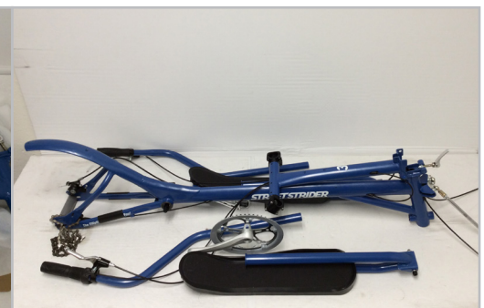
FIGURE 3.1.6 Once all the packing is removed, set the foot platform assemblies (lower pole, ski, foot platform, crank arm) aside.
