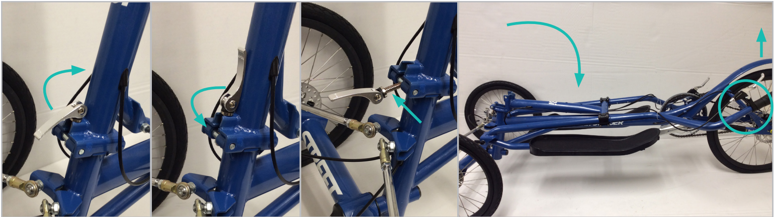
FIGURE 3.9.2 Lift the QR lever of the head tube fold joint up and rotate the stem forward. With one hand supporting the head tube, pull the QR stem to the right side so the pin disengages from the hole and lower the head tube down. With the rear brake locked, the StreetStrider can be lifted by the rear fender and rolled or stood up against a wall for storage.
