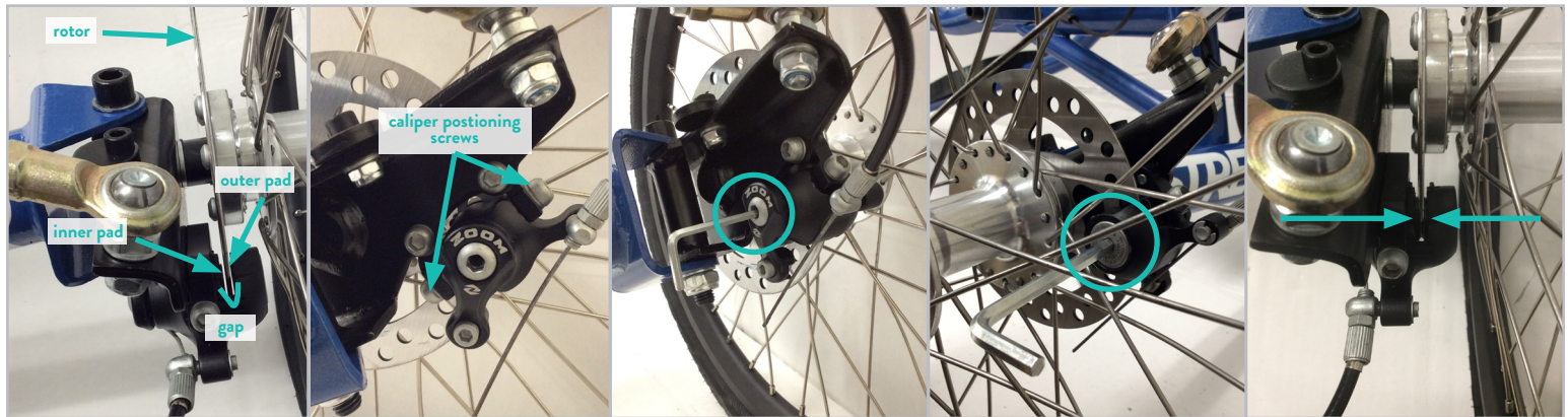
FIGURE 3.5.1 Make sure the brake rotor is centered in the caliper gap between the pads, and the wheel spins freely. If adjustment is needed, loosen the caliper positioning screws with a 5 mm hex wrench, tighten the inner pad with the 3 mm hex wrench inserted through the caliper lever, and the outer pad with the 5 mm hex wrench to center the rotor in the gap, then tighten the positioning screws. If the rotor is already centered in the caliper gap, tighten the pads against the rotor in order to attach the brake cable in the next steps.
