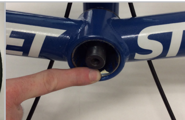
FIGURE 3.2.6 Grease the front bearing race in the front beam.
