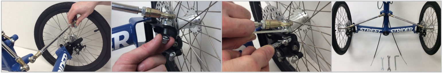
FIGURE 3.2.8 Lower the left steering linkage so the outboard rod end can be attached to the left steering knuckle.
