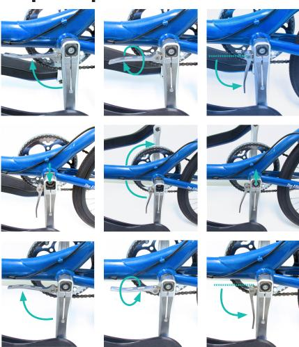
Rotate both crank arms to the 6 o'clock position, lift the QR lever on the left crank arm to the horizontal position, rotate the lever 180 degrees, and lower it to the left side of the crank arm.
