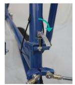
Raise the head tube while sliding the Quick Release (QR) clamp T-pin to the right. With the head tube in the full upright position, allow the QR clamp T-pin to insert into the hole. Rotate the QR stem to the vertical position so that the lever is against the head tube, then close the lever downward onto the shoulder.
