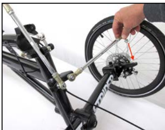
Figure 3.2.8 Lower the left steering linkage so the outboard rod end can be attached to the left steering knuckle.
