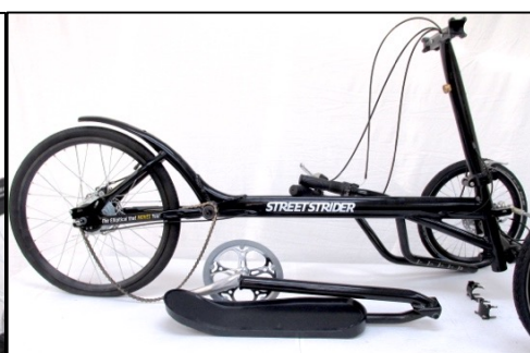
Figure 3.4.5 Retrieve the right foot platform assembly (lower pole, ski, foot platform, and crank arm with chain ring) and position next to right side of the frame. Make sure the chain is looped over the BB spindle.
