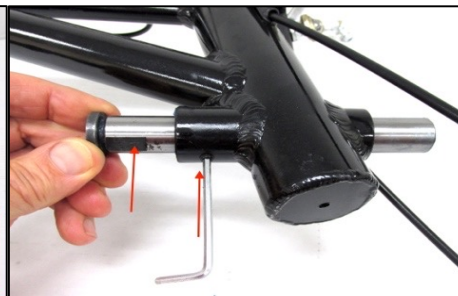
Figure 3.2.2 Loosen the set screw under the front beam shaft tube with a 3 mm hex wrench. Slide the shaft into the tube so that the flat section on the rear end of the shaft fits just above the 3 mm.
