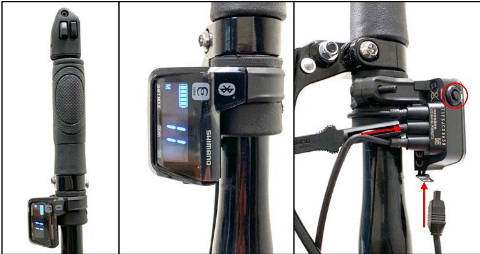
Figure 3.6.4 Top of right grip has thumb shifter buttons, left for upshift, right for downshift. Below rubber grip is system display that shows selected gear, level of battery charge, and shift mode. Parameters can be modified via blue tooth with Shimano E-Tube app.
