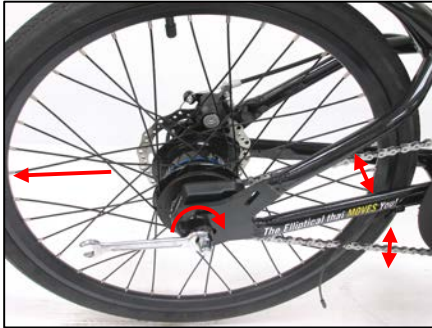
Figure 3.5.4 With the chain wrapped around both the right crank arm chainring and the rear hub sprocket, pull the rear wheel backwards to make the chain taut, center the front of the wheel in the frame chain stays, and tighten the acorn nuts with the 15 mm wrench, first right side then left. A taut chain should only move about 1/2" if lifted at a point midway between the chain ring and hub sprocket.
