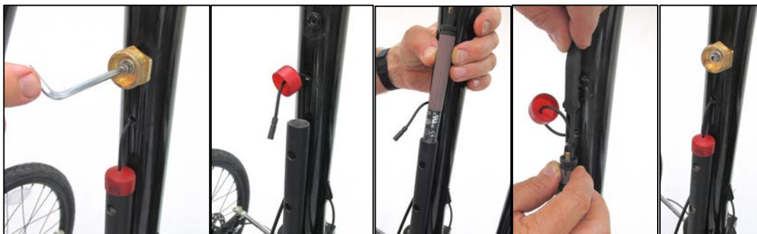
Figure 3.6.2 Using the 4 mm hex wrench remove the male brass strut connector from the head tube. Lift the plastic cap off the battery holder and pull the Di2 wire out of the holder.
