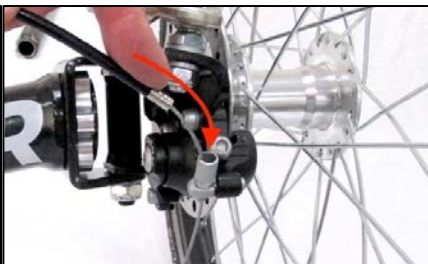
Figure 3.2.9 Unscrew the 13 mm nylon lock nut from the rod end stud, insert the threaded stud through the hole at the forward end of the steering knuckle, secure the stud with the nylon nut having one washer above and one washer below the knuckle and then hold the stud and tighten the nut using two 13 mm wrenches.
