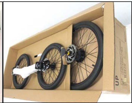
Figure 3.1.3 The front wheel assembly and rear wheel are the next 2 layers. Remove the wheels and set aside.
