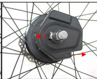
Figure 3.3.3 Replace the non-turn washer with tongue facing rearward and the Di2 cabling port facing forward.
