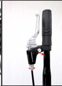
Figure 3.5.6 Both brake levers have a parking brake pin to hold the brake lever in a squeezed position. If the parking brake does not hold, unscrew the brake lever barrel adjuster.
