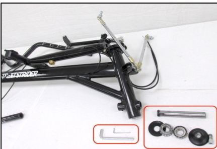
Figure 3.2.1 Lay the frame on it's left side. Retrieve the front beam shaft assembly, take the cap, tapered bearings and back plate off the shaft, and get the 8 and 3 mm hex wrenches.
