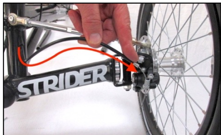
Figure 3.2.8 Lower the left steering linkage so the outboard rod end can be attached to the left steering knuckle.
