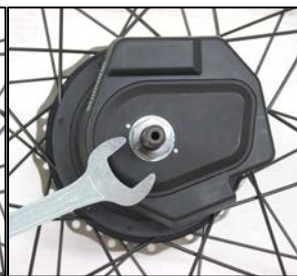
Figure 3.3.2 Retrieve the Di2 motor unit and 17 mm thin nut. Place the motor unit over the axle so that 2 silver dots are aligned with the red hub dots and the motor unit fits into the slots then secure with the 17 mm thin nut.
