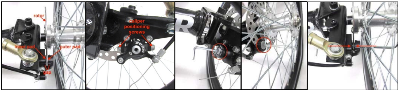
Figure 3.5.1 Make sure the brake rotor is centered in the caliper gap between the pads and the wheel spins freely. If adjustment is needed, loosen the caliper positioning screws with a 5 mm hex wrench, tighten the inner pad with the 3 mm hex wrench, inserted through the caliper lever, and the outer pad with the 5 mm hex wrench to center the rotor in the gap, then tighten the positioning screws. If the rotor is already centered in the caliper gap tighten the pads against the rotor in order to attach the brake cable in the next steps.
