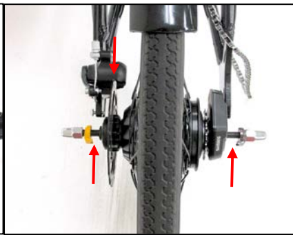
Figure 3.3.5 Unscrew acorn nuts on each end of the axle so there is an exposed section of axle under the non-turn washers that can slide into the dropouts. On the left side, align the brake rotor with the brake caliper gap.
