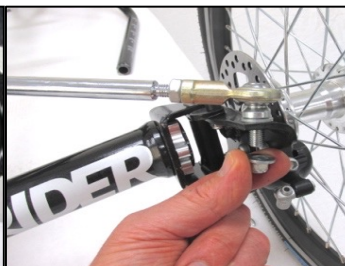
Figure 3.2.9 Unscrew the 13 mm nylon lock nut from the rod end stud, insert the threaded stud through the hole at the forward end of the steering knuckle, secure the stud with the nylon nut having one washer above and one washer below the knuckle and then hold the stud and tighten the nut using two 13 mm wrenches.
