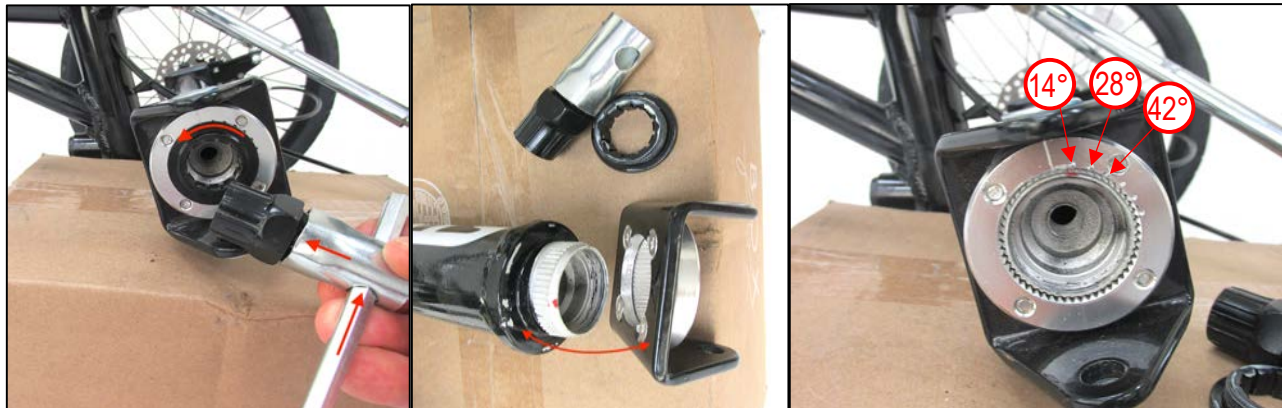
Figure 3.9.6 Use the clevis spline socket and the 19 mm socket with the 8 mm hex wrench as lever to unscrew the lock ring.
