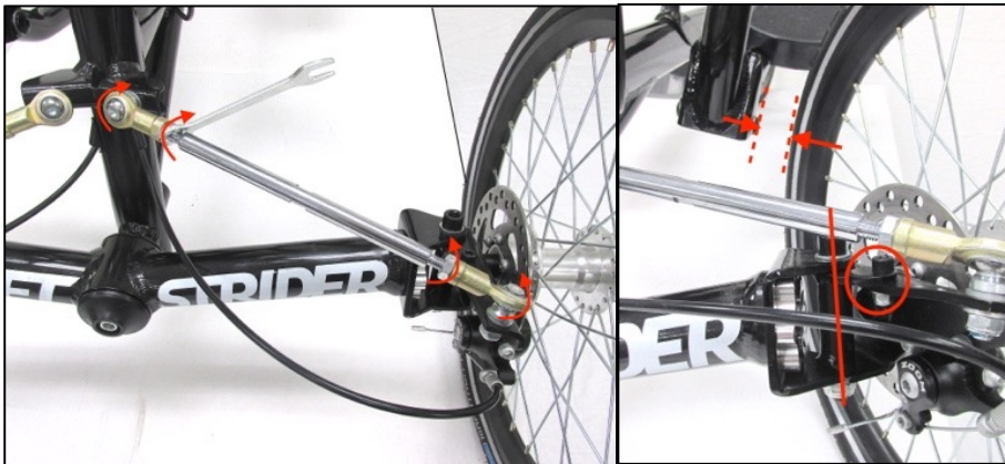
Figure 3.8.3 When the wheels are parallel to within 1/8" or 3 mm, tighten the jam nuts against the rod ends. To tighten the jam nuts, first rotate both rod ends as far as possible in the direction that the jam nuts will tighten, then use the 14 mm wrench to tighten the jam nut against the rod end. Check to make sure that each steering linkage rod is free to rotate as the StreetStrider is leaned to each side.
