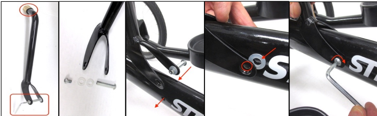
Figure 3.7.1 Retrieve the frame strut, which has a brass threaded collar at the top and frame saddle at the bottom. Using the 5 mm hex wrench, unscrew and separate the binding screw and the 2 nylon washers. Insert the longer female end of the screw through the hole at the end of the right side of the saddle and add a nylon washer on the inner side of the saddle. Align the saddle and screw with the frame hole and push the screw through the hole until it appears in the frame hole on the left side. Slide the second nylon washer between the saddle and the frame and over the screw end. Insert the male screw and tighten the screw with the 5 mm hex wrench. the receiver and tighten.
