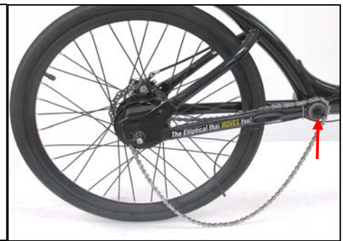
Figure 3.3.6 Slide axle into dropouts all the way forward, align the tongue of the non-turn washers with dropout slots, finger tighten the acorn nuts on both ends, and loop chain around hub sprocket and bottom bracket.
