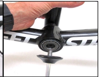
Figure 3.2.7 Insert the other bearing onto the shaft with the taper facing rearward. Put the cap over the front of the beam shaft, insert the 10 mm screw, and tighten with the 8 mm hex wrench.
