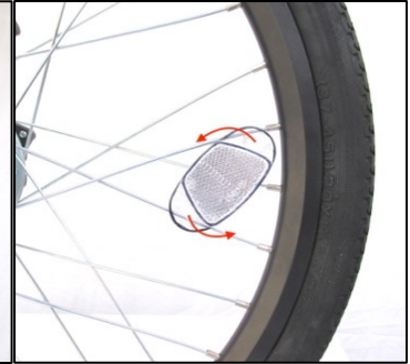
Figure 3.5.7 To install the 3 wheel reflectors onto the spokes, position the reflector between spokes and rotate so the reflector ends snap around the spokes.
