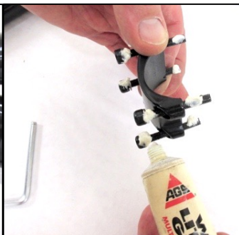
Figure 3.4.2 Apply a little grease to the screw heads and threads then set the caps with screws on the table.
