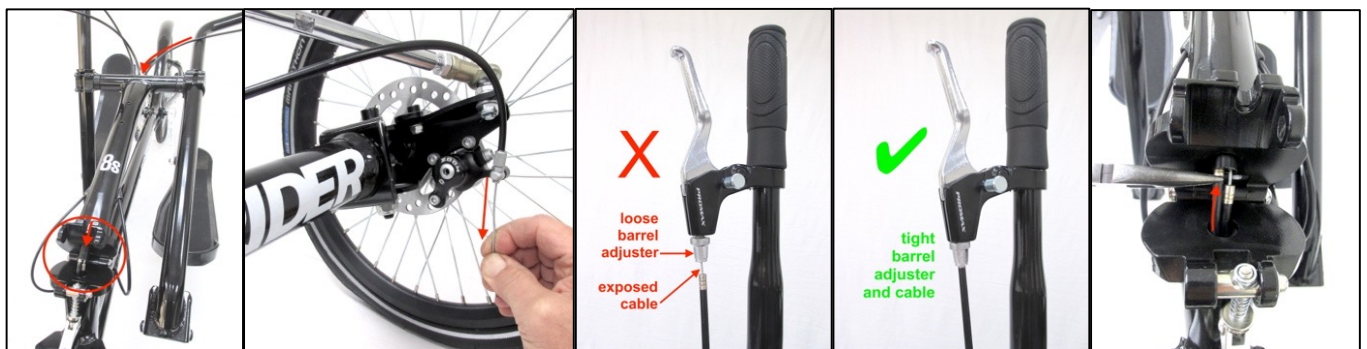
Figure 3.5.2 Fold the head tube down and push the cable housing from the left brake lever into the opening at the top of the crossbar so that the base of the cable doubler is visible through the hole in the fold joint. While pulling the cable down at the caliper make sure there is no exposed cable visible at the brake lever by inserting the cable housing ferrules into the brake lever barrel adjuster. Also, insert the cable housing ferrules into the base of the cable doubler using the pliers if needed.
