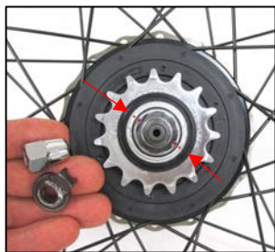
Figure 3.3.1 Remove the silver acorn nut and non-turn washer from the right axle end. Note the red dots aligned on the hub.
