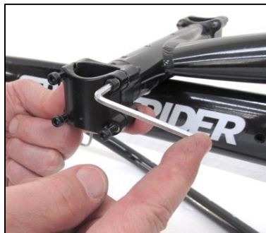
Figure 3.4.1 While the head tube is folded onto the main frame, use the 4 mm hex wrench to remove the 4 screws and caps from the both pole clamps at Joint #1.
