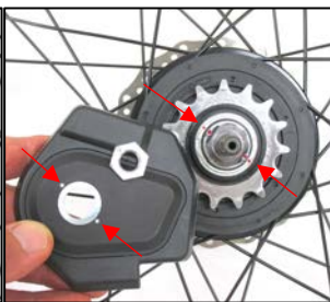
Figure 3.3.2 Retrieve the Di2 motor unit and 17 mm thin nut. Place the motor unit over the axle so that 2 silver dots are aligned with the red hub dots and the motor unit fits into the slots then secure with the 17 mm thin nut.
