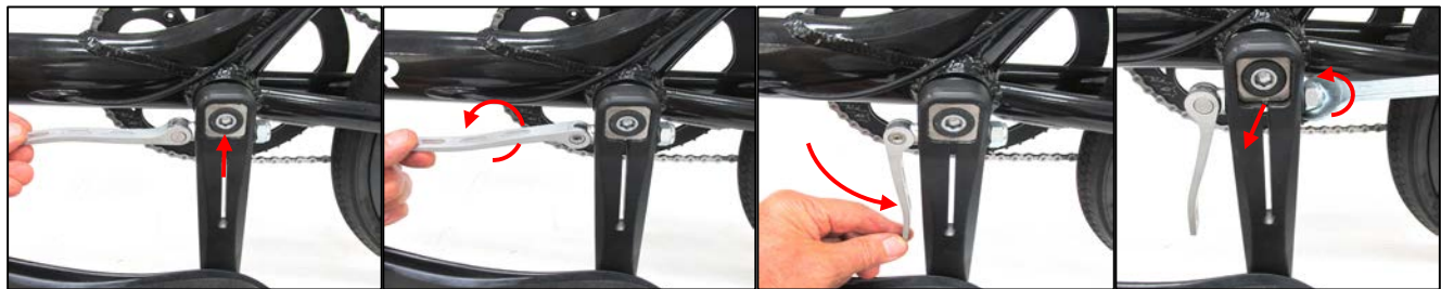
Figure 3.4.18 If the QR lever closes without any resistance open the lever, pull the crank arm off the BB ¼ inch (6 mm), tighten the 17 mm stem nut ¼ turn, push the crank arm back on, and close the QR lever. If needed, repeat until QR closes with some resistance.
