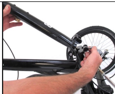
Figure 3.4.3 Raise the head tube while sliding the quick release, QR, clamp pin to the right. With the head tube in the full upright position allow the clamp pin to insert into the hole.
