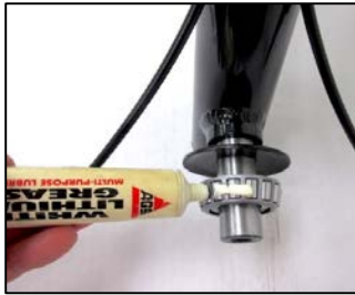
Figure 3.2.4 With the frame upright, slide the back plate and one of the tapered bearings, with taper facing forward, onto the shaft. Grease the bearings.
