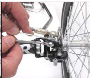
Figure 3.2.9 Unscrew the 13 mm nylon lock nut from the rod end stud, insert the threaded stud through the hole at the forward end of the steering knuckle, secure the stud with the nylon nut having one washer above and one washer below the knuckle and then hold the stud and tighten the nut using two 13 mm wrenches.
