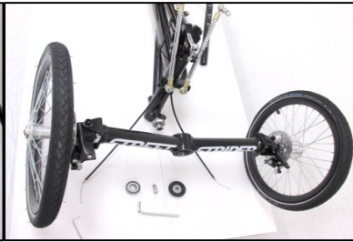
Figure 3.2.5 Unfold the front wheels on the front beam and set the front wheel assembly in front of the shaft.
